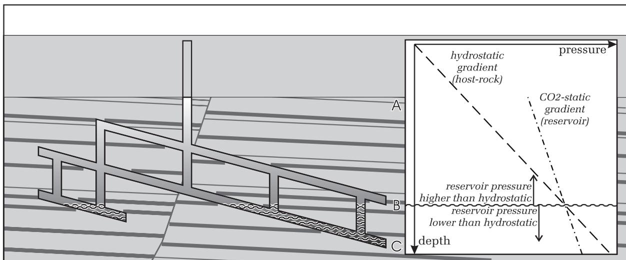
**Figure 3.** Schematic representation of a mine reservoir and the pressure evolution in the mine reservoir and the hosting formations. The reservoir is in overpressure relative to the hydrostatic gradient between points A and B, and in equilibrium with the hydrostatic pressure between B and C.
