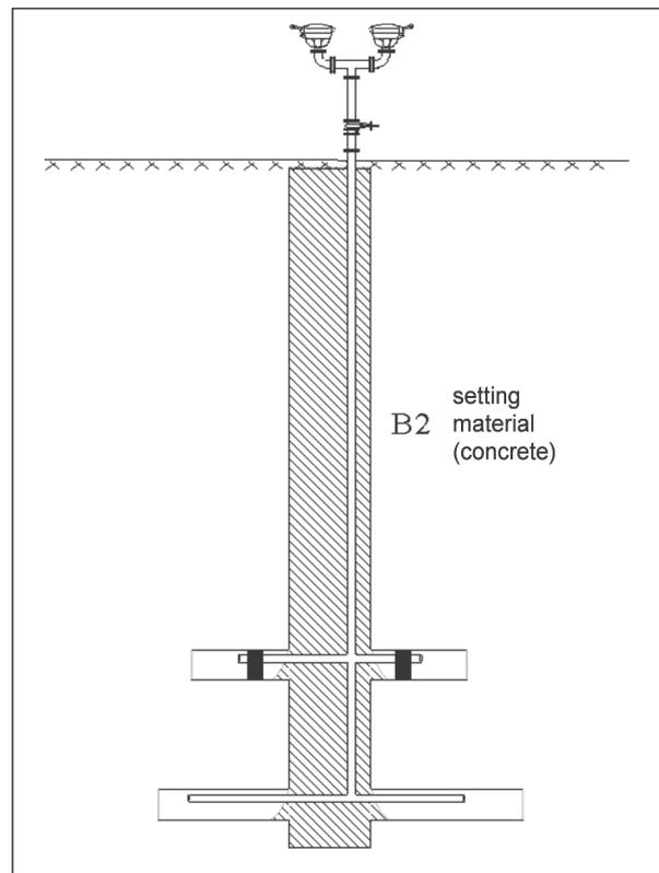
**Figure 4:** Complete filling of long-term stability with a degasification pipe.
