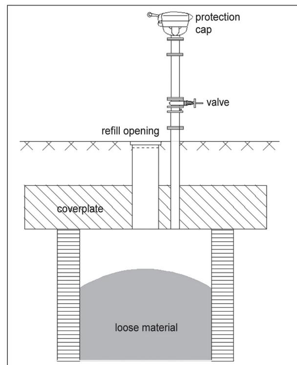
Figure 2: Shaft filled with loose material, closed with a coverplate and provided with a refill opening and a degasification pipe.
