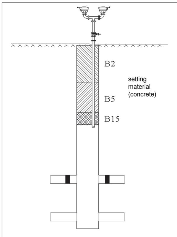
**Figure 3:** Partial filling of a shaft of long-term stability with a degasification pipe.
