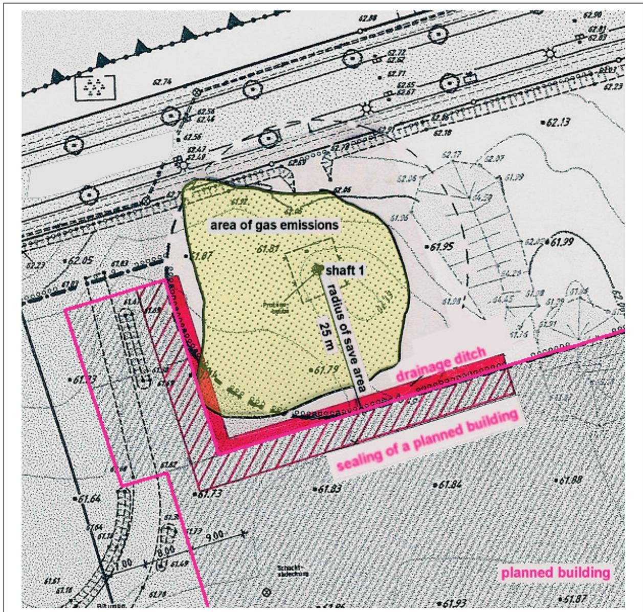
Figure 5: Area of gas emissions around an abandoned and filled shaft and protection of a planned building (Ickern).
