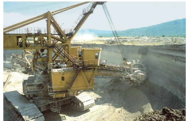
**Figure 9.** Bucketwheel Excavator cutting overburden at Gacko Mine.
