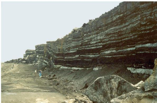
**Figure 6.** Ten metre highwall showing lignite with numerous light coloured calcareous interbeds, Gacko Mine.
