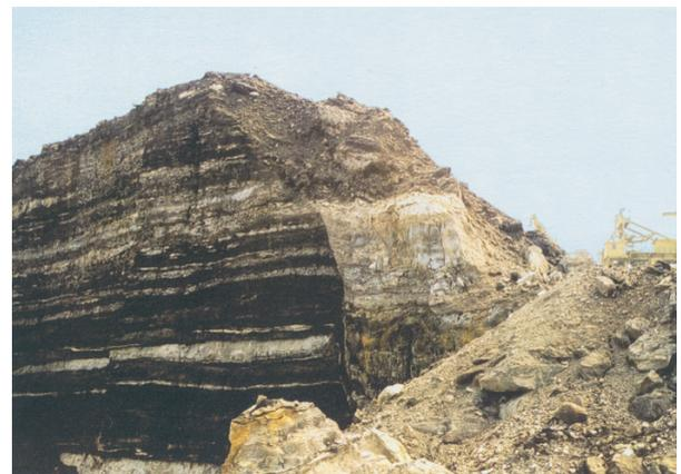
**Figure 3.** Fault downthrowing overburden on the right against banded lignite on the left of the photograph, producing highwall termination. Height of face 10 metres.
