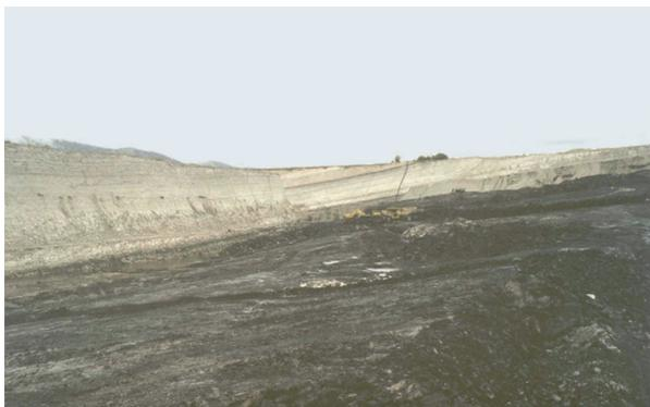
**Figure 2.** Lignite and light coloured overburden dipping at 7° to southwest, Pit B, Gacko mine.
