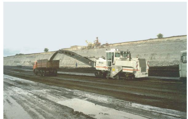
**Figure 10.** Wirtgen Machine stripping lignite in Pit B, Gacko mine.
