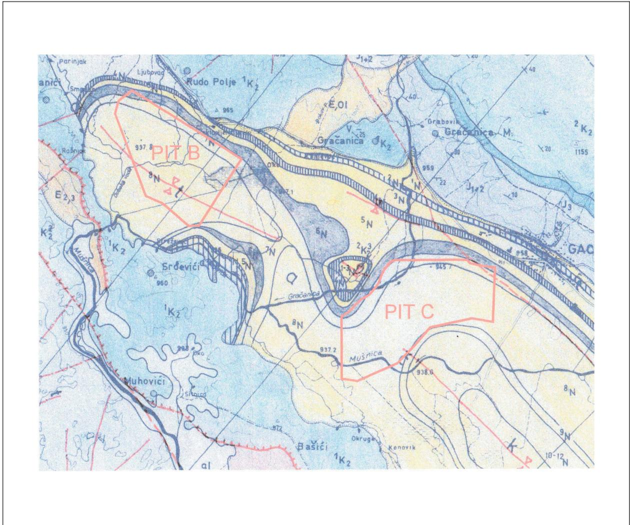
**Figure 1.** Geological Map of the Gacko Basin, showing folded Tertiary sediments (yellow) surrounded by Cretaceous limestones (blue). The main lignite seam (grey) and two subordinate lignite seams (striped) are preserved along the northern limb of the syncline (produced by Gacko Mine & Power Company). Map Scale 1:25,000.
