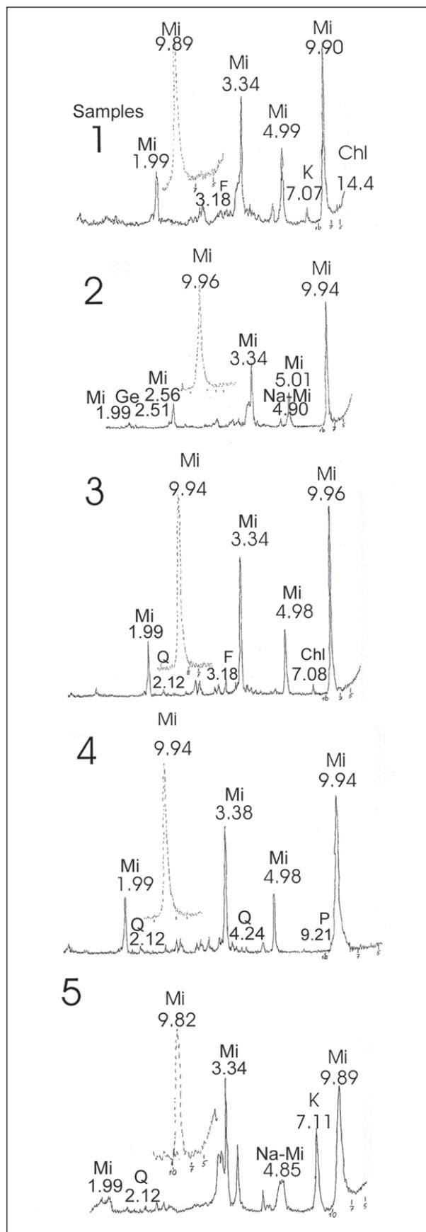
Figure 4. XRD patterns of the pelitic rock fractions of the Dombarovsk deposits.
