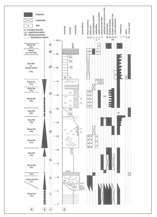
**Figure 2.** Sedimentological log of the Lambert quarry (Upper Pragian). a: interpretation of the paleoenvironments, b: vertical evolution of grain size, c: succession of lithological units, d: columnar lithological section, vertical distribution and abundance of sedimentological features.
