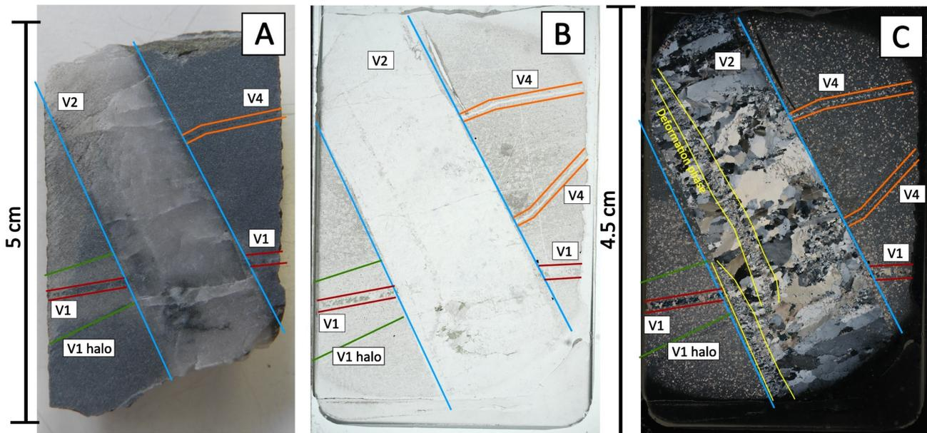
**Figure 6.** Sample IC211M02 (S1 at a depth of 61.5 m), rock sample and thin section under PPL and XPL, illustrating the occurrence of three vein generations and alteration halos.
