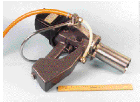
Figure 4. Pneumatically operated concussion stunner (Fa. Schmid & Wezel, Maulbronn, D).
