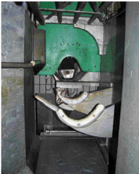
Figure 3. Multifunctional stunning box (looking in the direction of the animal) with muzzle electrode (middle in the front), green head fixing slide (in down-position, with integrated neck electrodes), brisket- (with heart electrode) and abdomen-support-bars (Fa. BANSS; Biedenkopf, D).
