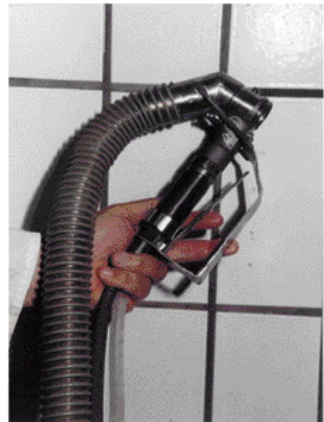
Figure 7. Pneumatically operated round knife, with rotating blade and hose for vacuum sucking (Fa. EFA; Maulbronn, D).
