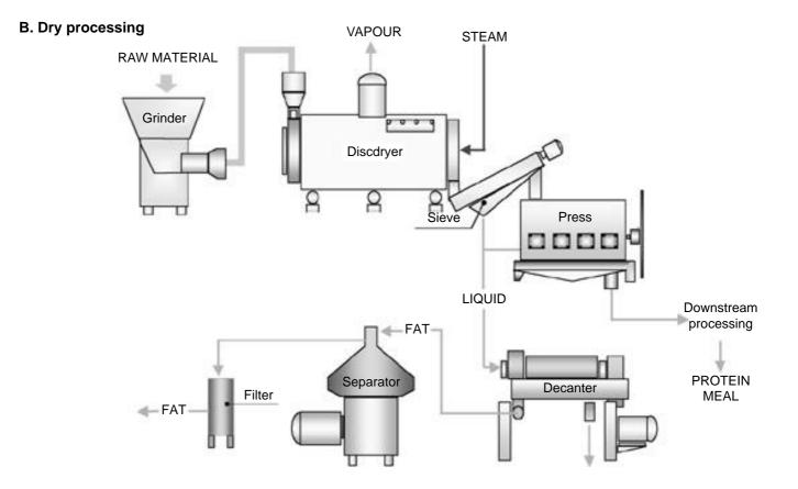
Figure 3. Schematic diagrams of two rendering processes.
