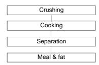
**Method 2.** Atmospheric/natural fat/batch. Where necessary, the material is reduced in size by crushing. It is then heated *in a steam-jacket vessel (often with a steam-heated rotor)* to remove the inherent moisture. The moisture is driven off as water vapour at atmospheric pressure. After drying/cooking, the material is then separated into its liquid/tallow and solid/protein fraction, normally by mechanical means before being made into animal protein meal by milling.
