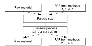
**Method 1.** Pressure/batch or continous. Applied to mammalian material either as a "pre" pressure process (raw material) before entering any one of methods 2–5 or it is applied as a "post" pressure process after completion of any one of the methods 2–5.
