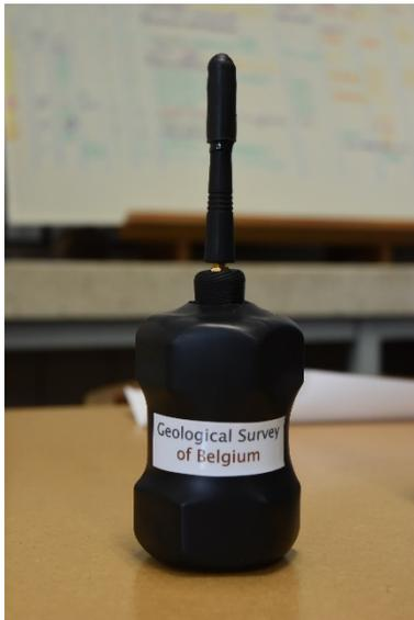
**Figure 2.** NiphNet node, as a wireless Niphargus inside a waterproof, stainless steel container.
