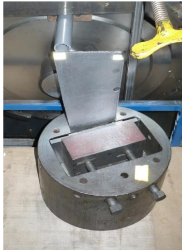
Fig. 27: Blade mounted onto a block with the nozzle of the exciter at the top-left corner
