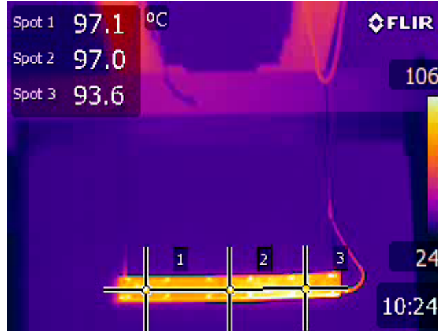
Fig. D.1: Picture from the IR camera taken a few seconds before tapping the beam to measure its behavior at elevated temperatures. Compare to Figure 1a. The bright spots appearing in a grid should be ignored, as they correspond to locations that were marked with black ink (see Figure 1b), suggesting that the ink affects the emissivity of the surface.
