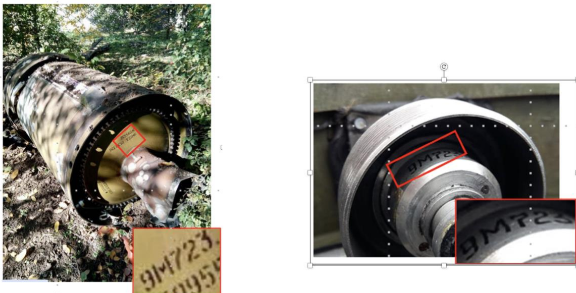
Figure 19. Examples of the 9M723 marking characteristic of Iskander M series missiles. On the left: Open Source Munitions Portal ( https://osmp.ngo/osmp4/ ); on the right: "Azerbaijan claims Armenia used Iskander missiles to destroy the city of Shusha", March 31, 2021, Haqqin.az (< https://haqqin.az/news/205714 >).
