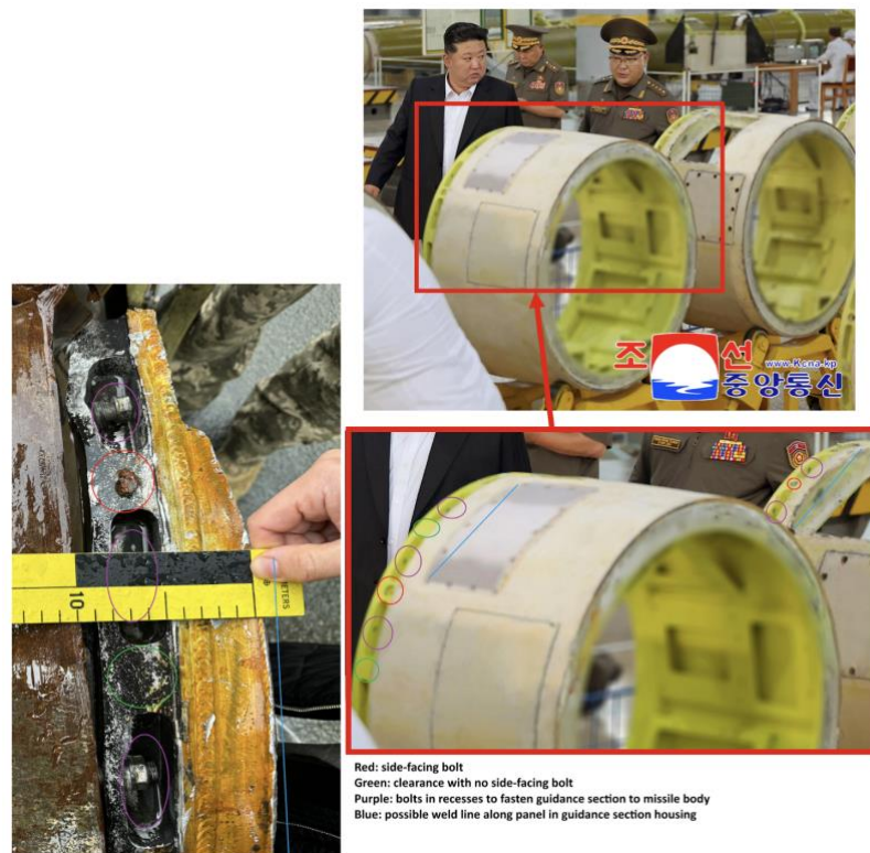
Figure 14. On the right, images published in September 2025 of the guidance section housing of Hwasong 11 series missiles. On the left, an image of the remains of the housing seen during the inspection in Kyiv. Common to both images, as indicated by colored circle. Source: author's image (left); KCNA (right).
