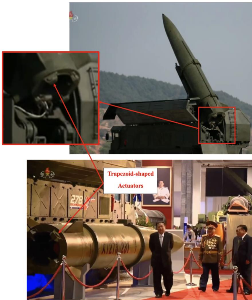
Figure 10. Trapezoid-shaped actuators seen in published images of the Hwasong 11 (KN-23). Note the absence of other mountings on the base of the missiles. Source: KCTV.
