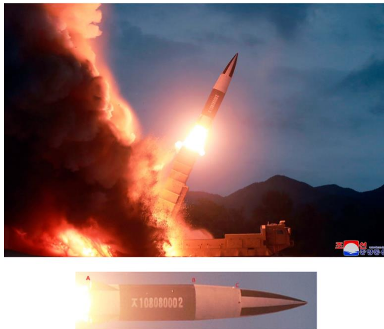
Figure 5. Top: Launch of a Hwasong-11B missile (Source: KCNA). Bottom: Enlarged image of the missile. If we assume that the diameter of the base of the missile (point A) is 110 cm (as measured by the Panel experts in Kyiv) and that this diameter remains constant along the length of the missile's body to point B (as indicated in Figure 4), then based on the proportions of this image the diameter of the forward end of the engine (point C) is about 91.2 cm. Within the margins of error of this exercise this diameter is equivalent to that estimated by the experts, based on their measurements (92cm).
