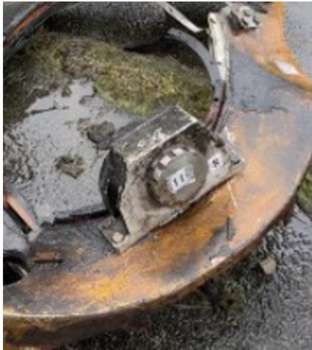
Figure 9. Trapezoid-shaped actuator attached to the base of the missile inspected in Kyiv. The base had no other attachments. Source: authors' image.
