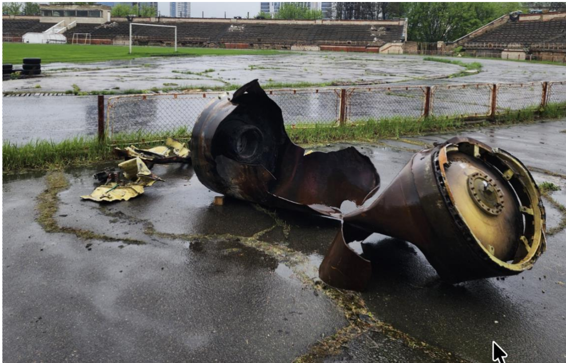
Figure 1. Missile airframe debris laid out by Ukrainian authorities for inspection by Panel experts. The front end of the engine (to the right), the rear end of the engine (to the left), and related components scattered on the ground further to the rear constituted the majority of the debris. The warhead would have been located on the front end of the engine. Source: authors' image.
