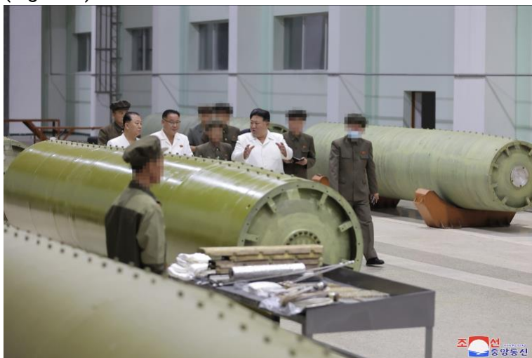
Figure 6. The forward end of Hwasong 11 series missile bodies, with their eight connection yokes. Note cable-duct fixings running along the length of the top surface. Source: KCNA.
