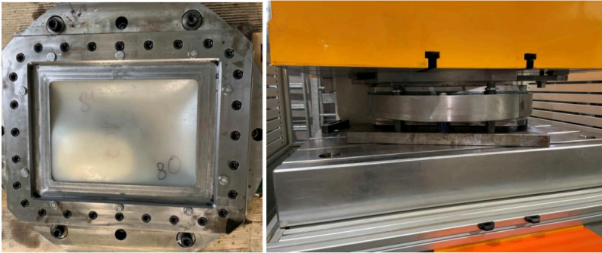
Fig. 5. The forming tool assembled with the diaphragm with an elastomeric plate (the left figure presents an open tool and the right figure presents the tool set on a hydraulic press).
