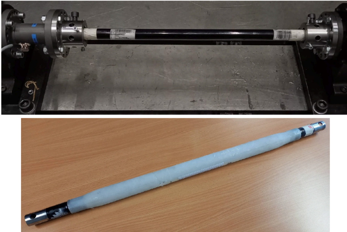
Fig. 12. (top) Test set-up with an original steel sample; (bottom) a glass fibre composite sample
