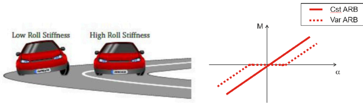
Fig. 2. Low and high roll stiffness (right) [1] and progressive stiffness with torsion to improve comfort around the center point (left), allowing a compromise between comfort and handling.
