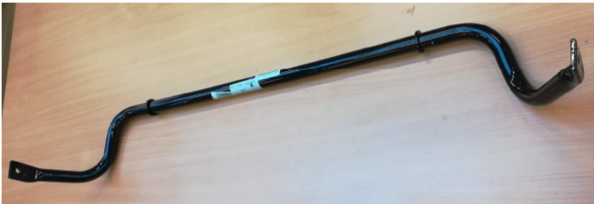
Fig. 3. Front ARB of an Audi A6.
