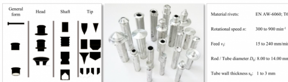
Fig. 2. A number of samples of general shapes and local part geometries of possible FSJCs (left); a selection of different realized part geometries produced with the help of friction-spinning (centre); used parameter range (right).
