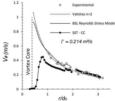
Figure 8 - Tangential velocity profile for  $z/H_{in} = 0.26$
