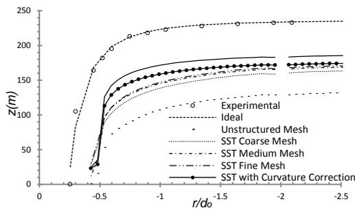
Figure 5 - Sensitivity analysis for the solution of the water surface profile
