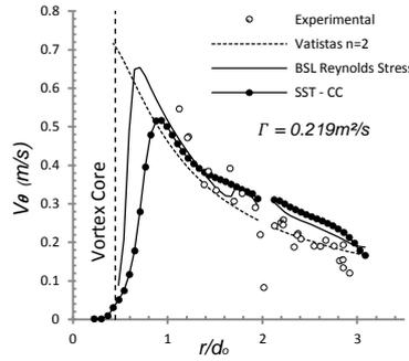
Figure 9 – Tangential velocity profile for  $z/H_{in} = 0.56$
