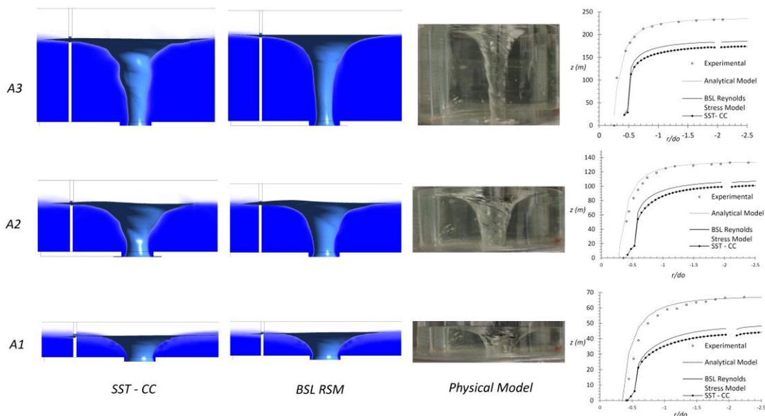
Figure 7 – Summary of comparative analysis for water surfaces between the analytical, SST-CC and RSM physical model for A1, A2 and A3 test cases.
