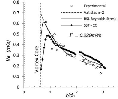
Figure 10 – Tangential velocity profile y  $z/H_{in} = 0.75$
