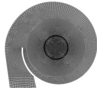
Figure 4 - Plan view of radially structured mesh
