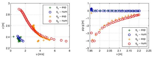
Figure 6 - Horizontal velocity profile at crest (left) and pressures on the bottom (right)
