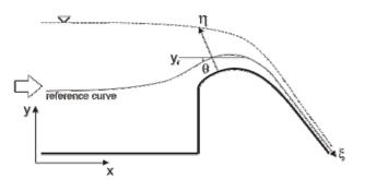
Figure 2 – Curvilinear coordinates for a spillway
