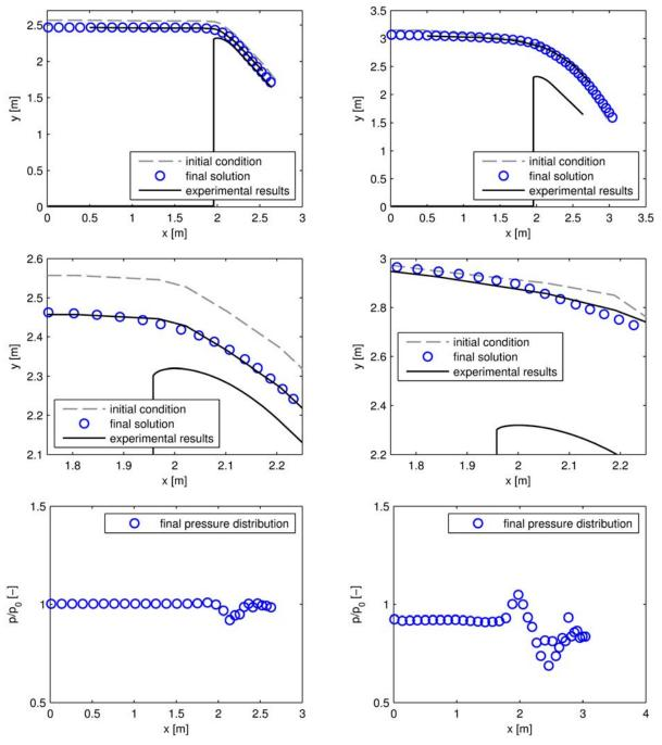
Figure 5 – Free surface position and pressures for a spillway flow (left:  $q=q_1=0.1275m^2/s$ ; right:  $q=q_2=1.7632m^2/s$ )
