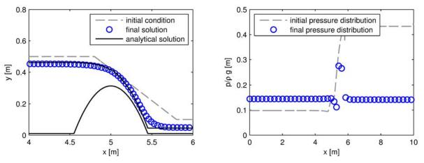
Figure 4 – Test case (c): transcritical flow over a parabolic bump
