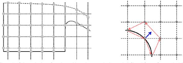
Figure 1 – Schematic view of regular and irregular zones in the mesh (left) and Green-Gauss principle (right)
