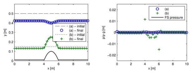
Figure 3 – Test cases (a and b): subcritical (a) and supercritical (b) flows over a parabolic bump (plain lines are for analytical solutions)
