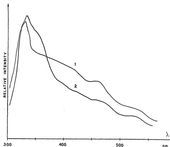
Figure 2.- Fluorescence spectra of gypsum from Betekom (1) and Tongeren (2) with a relative intensity of 90 and 30 respectively.
