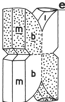
Figure 1.- Cruciform penetration twin of gypsum according to (100) b(010); m(110); l(111); e(103).
