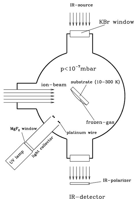
Figure 1: Schematic depiction of the experimental set-up.
