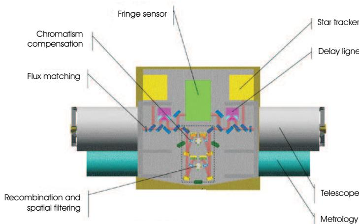
Figure 3: Payload located in the central satellite. The detection/spectroscopy unit is located on a second stage, which is fiber-linked to this stage.
