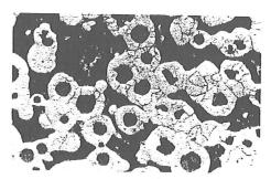
Figure 1. Microstructure of nodular cast iron 400-12, magnification 100x.
