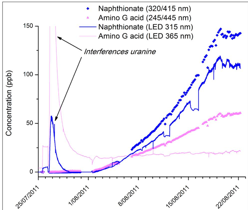
**Figure 7.** Variations of fluorescence background signal (LED 365 nm) due to natural organic matter in a karst spring giving rise to apparent fluctuations of approximately 7 ppb of amino G acid.
