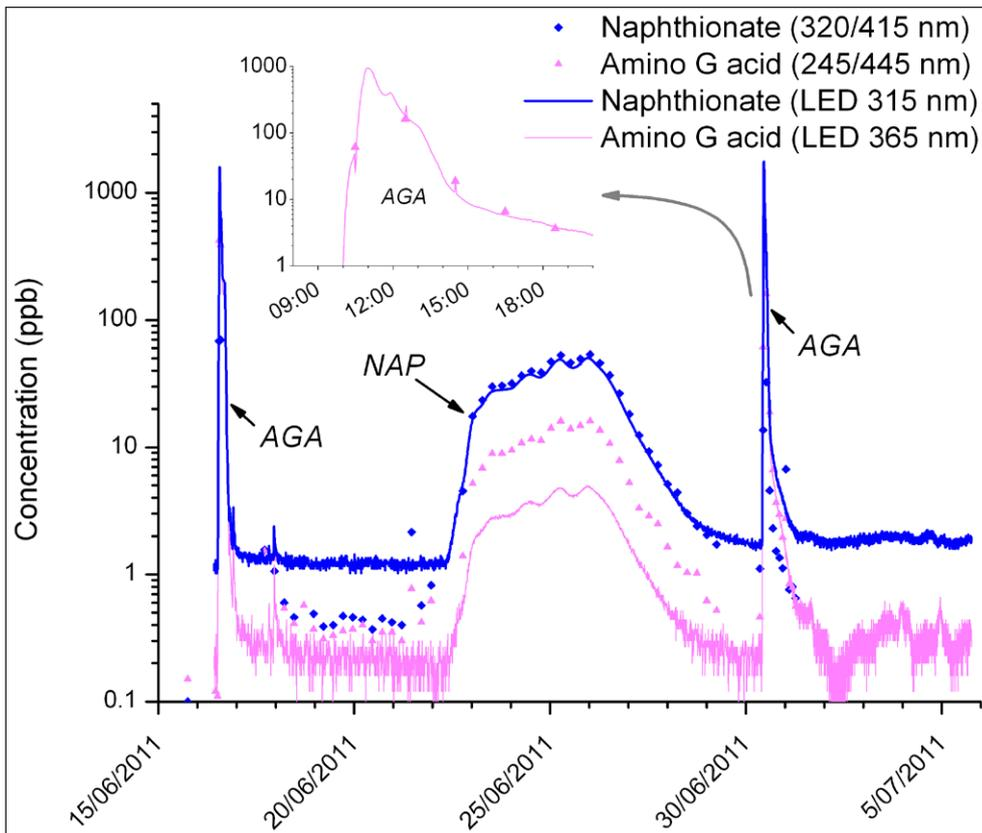
**Figure 5.** Breakthrough curves (logarithmic scale) of NAP and AGA in a sandy aquifer as inferred from field fluorometer signals (LEDs 315 and 365 nm) combined with laboratory spectrofluorometric data at optimal EX/EM wavelengths.
