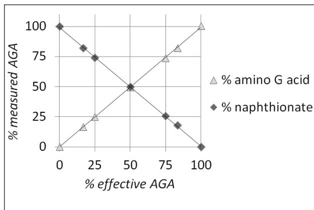
**Figure 3.** Identification of NAP and AGA mixed in different proportions in laboratory solutions, using the fluorometer equipped with LEDs at 315 nm (NAP) and 365 nm (AGA) and with a built-in resolution algorithm.
