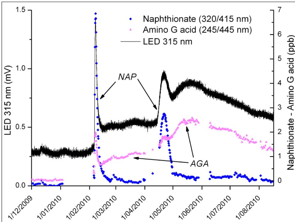
**Figure 4.** Breakthrough curves of NAP and AGA in a karst aquifer as inferred from the field fluorometer signal (LED 315 nm), compared to laboratory spectrofluorometric data at optimal EX/EM wavelengths.
