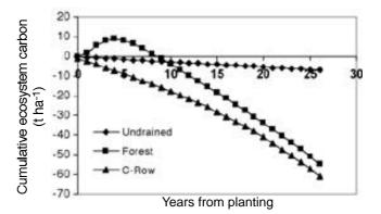
**Figure 2.** Cumulative C-exchange following drainage/ afforestation of peatland in SW Scotland. Year 0 represents the undrained state, drainage/planting is assumed to take place on the first day of year 1. The output from the C-Flow model simulates a 90% *Picea Sitchensis* (Bong.) Carr and 10% *Pinus contorta* Douglas mixture on a mineral soil.
